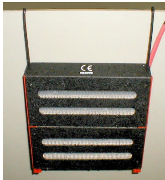
Fig. 3: Polaris Modular installed vertically in tank showing safe liquid level
