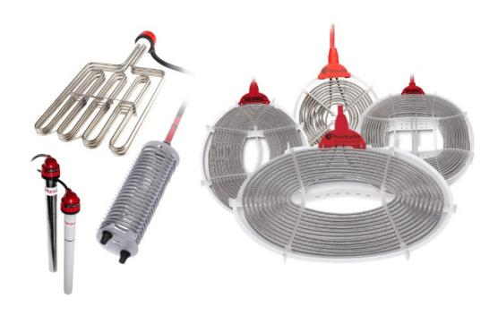
The Polaris Popular fluoropolymer immersion heaters are designed for use where aggressive chemicals need to be heated to temperatures up to 100°C. All heaters have optimum chemical resistance against corrosion caused by chemicals such as nitric, hydrochloric, sulphuric and hydrofluoric acids, and are inert enough to be used where non-contamination is a requirement.
