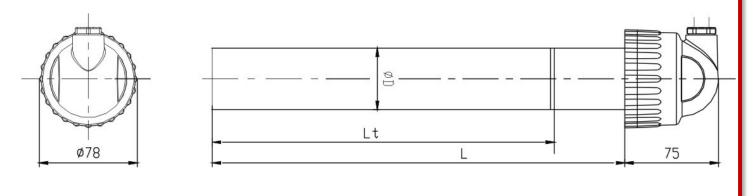
The heaters are designed to be mounted vertically in the tank and will occupy the minimum amount of space. The heater should be mounted on the flange of the tank using the optional hanging bracket. It should be position so the hot zone of the element (marked on the casing) is always below the liquid. It is available in sizes 1 kw to 4.5kw in single or three phase with a head to IP65 and flying lead for easy connection leaving no exposed joints near sur-
